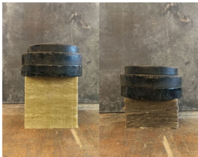
Figure 5. Stone wool samples before (left) and after (right) mass-loss experiment with a weight of 5 kg on top. [Colour figure can be viewed at wileyonlinelibrary.com ]
