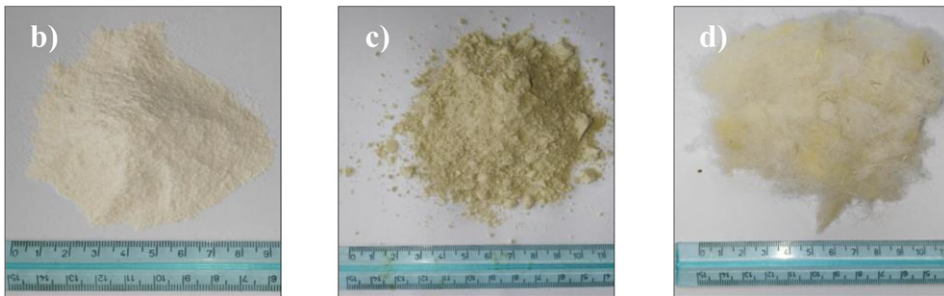
Figure 1. Aggregates and natural fibers. (a) Grain size distribution of calcareous sand and zeolite. (b) Calcareous sand. (c) Zeolite. (d) Wool fibers.
