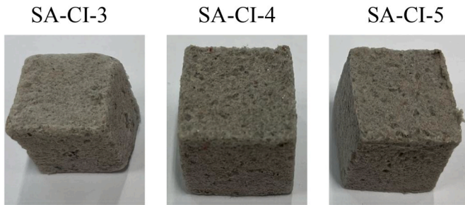
Fig. 4. Dried samples of the optimized composition of silica aerogel/bio-based materials composites.
